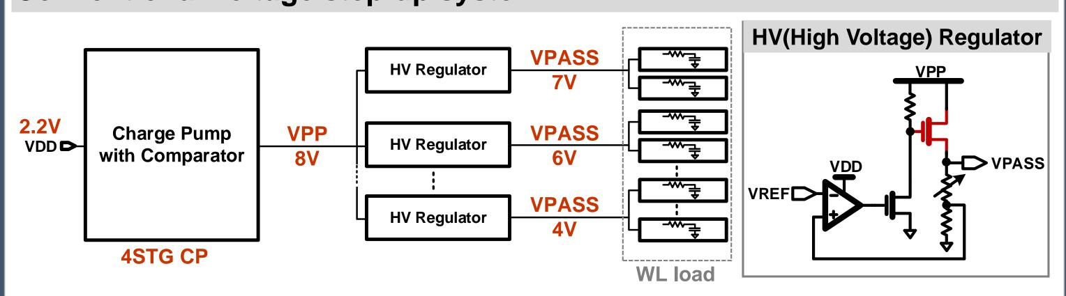
The regulator output uses NMOS. VPP must be sufficiently higher than the VPASS voltage.
